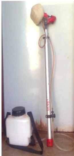
Micron ulva + spinning disc sprayer showing water tank and spraying mechanism
